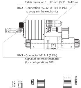
KN1 - Main input connector M23 (7 PIN)
