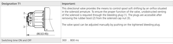
The switching times shown are valid for viscosity  $v=32~\text{mm}^2/\text{s}$  (156 SUS) and nominal voltage. They depend on working pressure and flow rate of the directional control valve.
