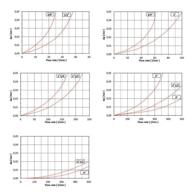
N.B. The above diagrams have been obtained at the FILTREC laboratory, according to the ISO 3968 specification, with oil having viscosity 32 cSt and density 0,875 Kg/dm<sup>3</sup>.
