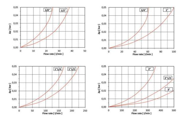
N.B. The above diagrams have been obtained at the FILTREC laboratory, according to the ISO 3968 specification, with oil having viscosity 32 cSt and density 0,875 Kg/dm<sup>3</sup>.
