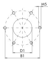
TANK MOUNTING PATTERN (DIN 24557/2)
