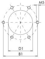
TANK MOUNTING PATTERN (DIN 24557/2)
